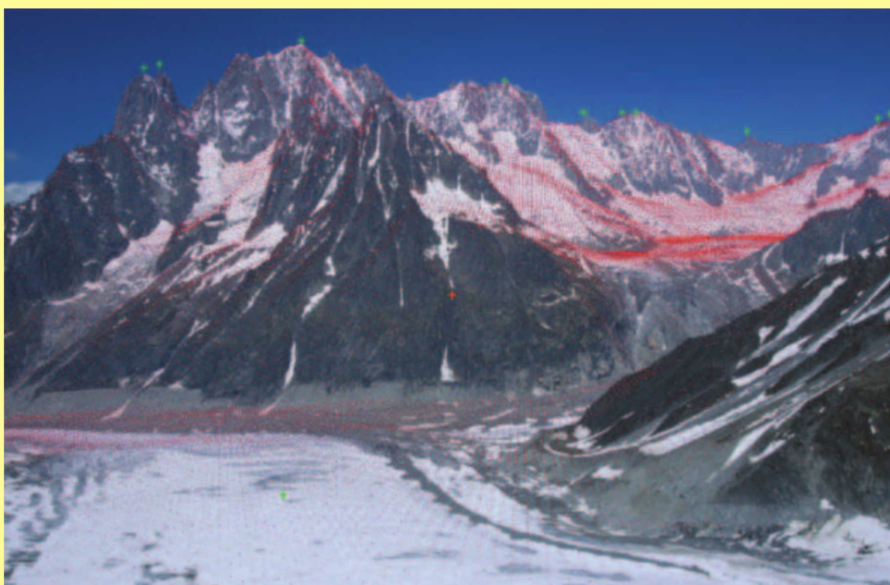
Figure 4: Superimposition of the perspective projection of a DEM of the Mer de Glace over a photograph of the area. Red dots are the perspective projections of the original DEM grid cells, and green dots are the ground control points (GCPs). (Corripio, 2004)
