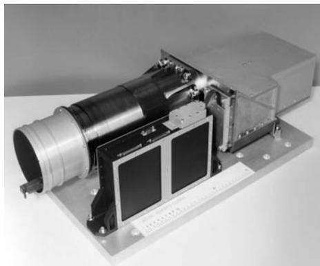
Figure 3: The Compact High Spatial Resolution Imaging Spectrometer (CHRIS), currently orbiting on the agile PROBA-1 satellite. Photograph courtesy of Sira Electro-Optics Ltd.
