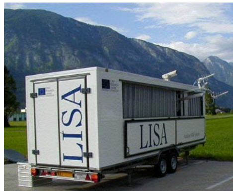
Figure 3. The mobile SAR system LISA of JRC-IPSC below Eiblschrofen.
