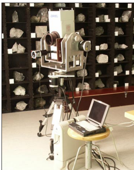
Figure 2. FieldSpecFR combined with Oriel 1000 W illuminator was used to 'scan' the shelf, which was loaded by rock and environmental samples. The white standard reflectors (6x6 cm) were placed near to the samples in order to ensure spectroradiometric corrections after possible instrumental drift.
