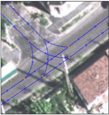
Figure 3. A 3-arm junction overlaid with the lane level model
