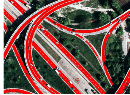
Figure 8. Supervised classification for a junction with pixel intensity and texture parameters (background image: color orthophoto)
