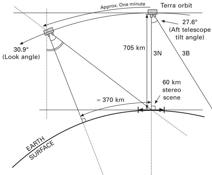
Figure 2. Diagram of the Aster recording geometry [6].
