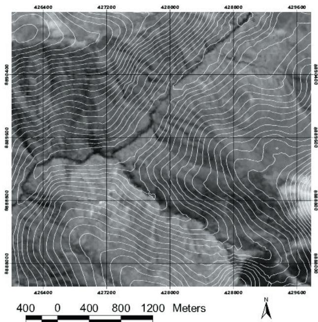
Figure 4. Detail of the Orthomosaic with contour lines each 50 m.
