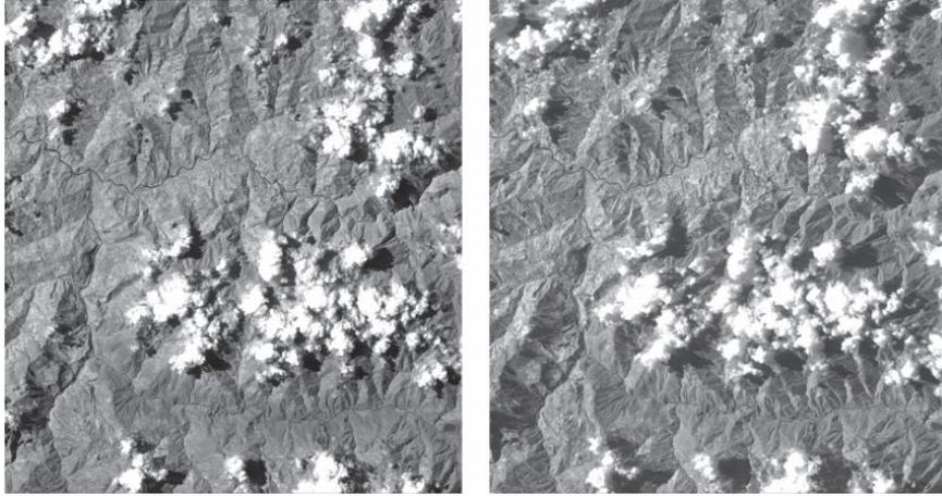
Figure 1. Stereo pair of aster 3N (left) and 3B (right) images.
