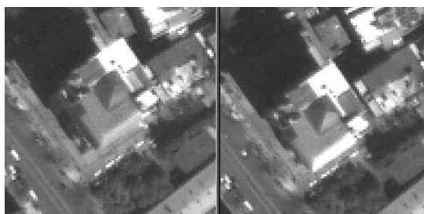
49 m high building in IKONOS stereo model with height to base relation of 7.5
