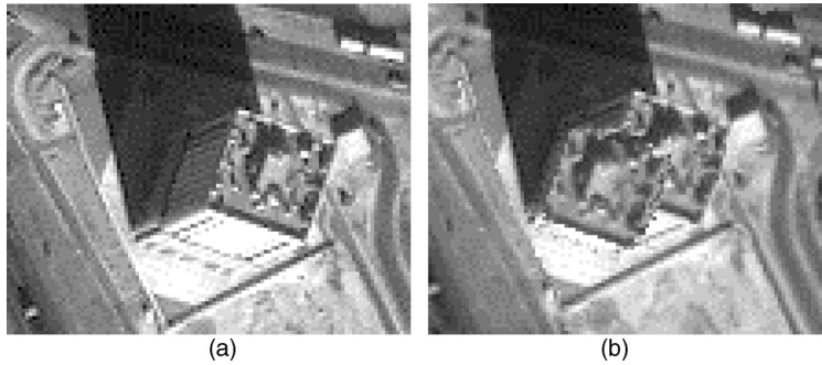
Figure 3. (a) sample of the original Ikonos showing a tall building; (b) the same image after rectification with the DSM. The top of the building appears twice.
