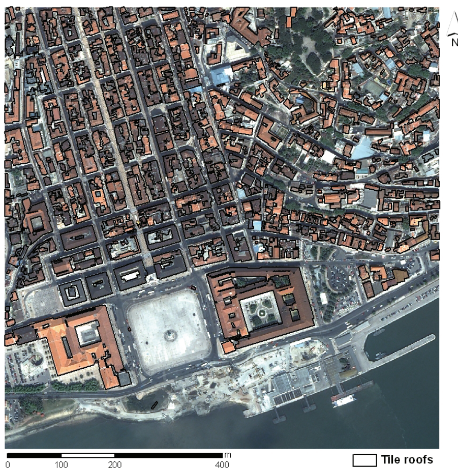
Figure 2. Example of extracted features in study area A-Baixa.
