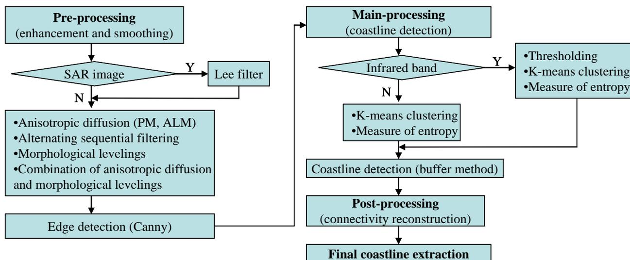
Figure 1: The methodology for coastline detection from remotely sensed imagery, based on advanced smoothing techniques and the Canny edge detector.
