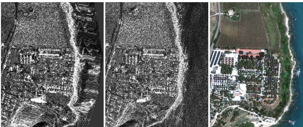
Figure 6: Left: orthorectified image -product COSMO-SkyMed © ASI (2011), Center: source image (reprojected without DEM to facilitate comparison) -product COSMO-SkyMed © ASI (2011) and Right: optical image of the same area © Google Earth optical image. The shoreline can be easily traced on the reprojected image, whereas in the case of the orthorectified image there appear to be artifacts.
