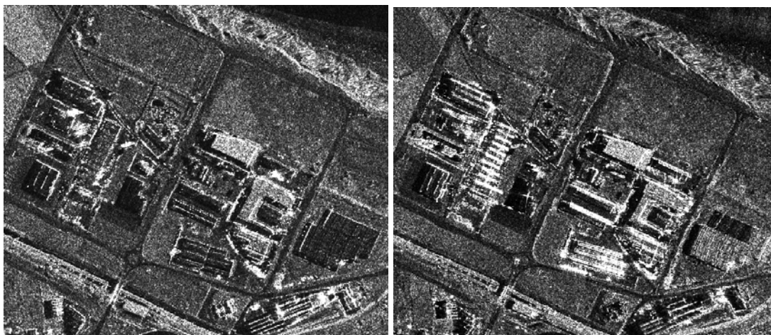
Figure 3: Left: COSMO-SkyMed acquisition taken in Right-Ascending mode -product COSMO-SkyMed © ASI (2011). Right: The same areas imaged by a COSMO-SkyMed acquisition in Right-Descending mode -product COSMO-SkyMed © ASI (2011). Differences in the illumination of walls/roofs and fields are evident. The dune system (white area in the upper section of the images) does not seem particularly affected by the change in illumination direction, probably due to its roughness.
