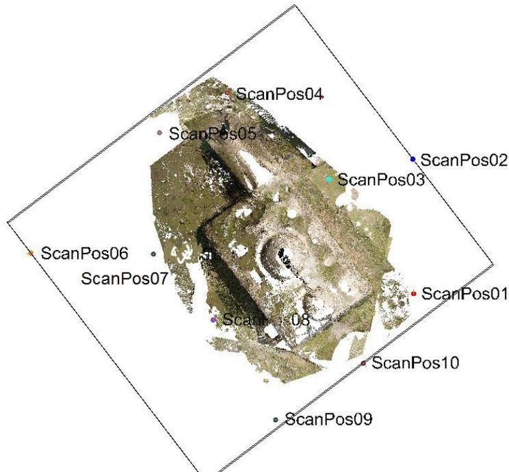
Figure 3: Scan position for external wall of bath.
