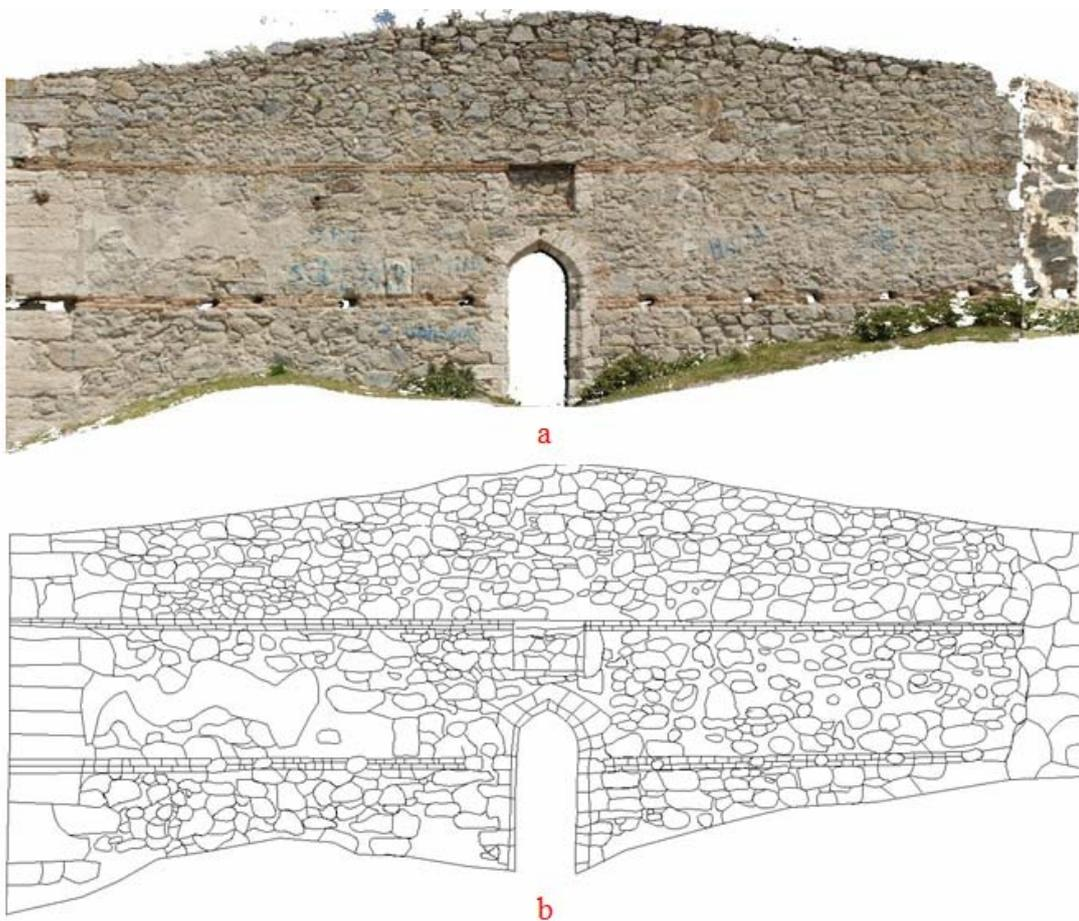
Figure 5: a: orthophoto image of front wall of the bath; b: 2D CAD drawing of front wall on orthophoto image.
