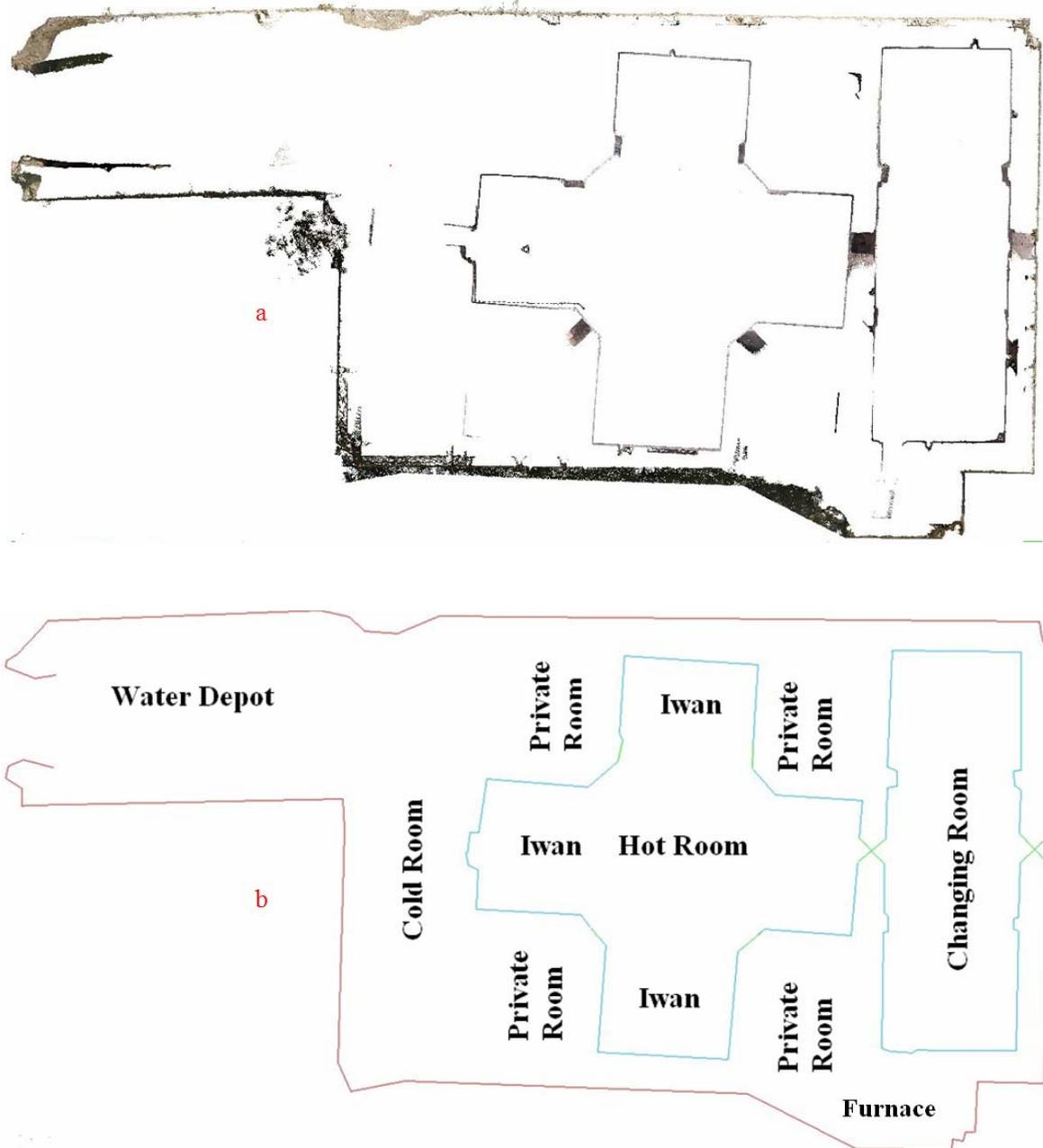
Figure 6: a: Plan view of point cloud bath; b: 2D plan drawing of bath on point cloud.
