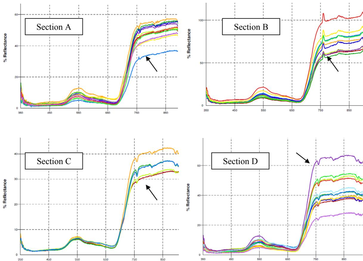
Figure 8: Spectro-radiometric measurements in 05/03/2010. Each diagram corresponds to a cross section (A-D) while the spectral signature indicated with an arrow corresponds to the subsurface geophysical anomaly [15].
