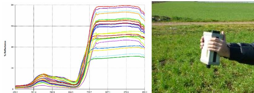
Figure 12: Spectral signature profiles over a magoula (left) and photo during the field campaign using the GER 1500 spectroradiometer (right).
