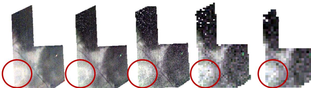
Figure 2: Crop mark (Nikaia 16 site at the Thessalian plain) in circle in different scale resolution (1m, 2m, 4m, 10m, 15m and 30m pixel resolution from left to right).
