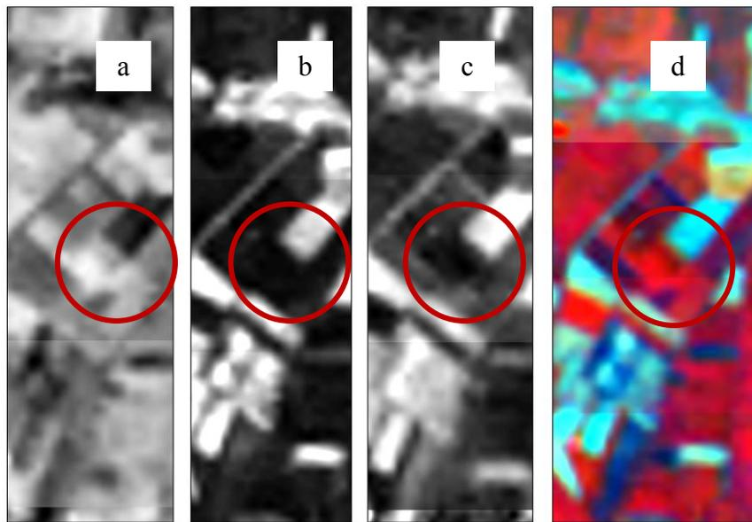
Figure 19: Tasseled Cap results for Almyros II site (in red circle), (a) Brightness, (b) greenness, (c) wetness and (d) RGB of the first three components of the T-K algorithm.
