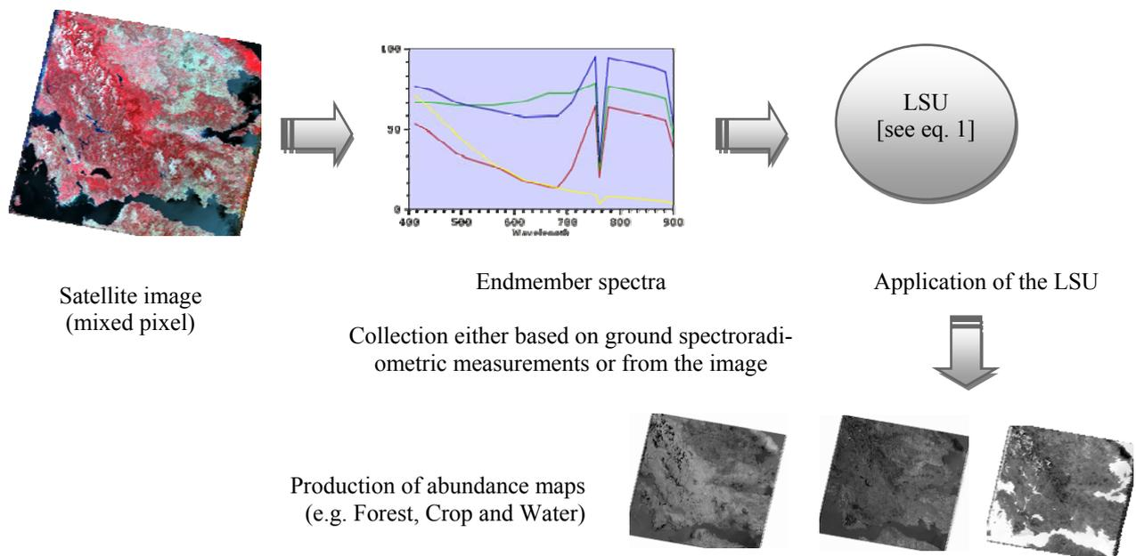
Figure 3: Methodological diagram for the application of the LSU algorithm.
