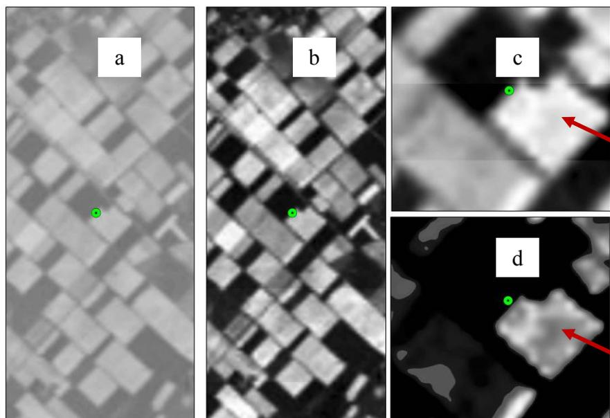
Figure 16: NDVI results for Prodrornos II site (in green circle). (a) Raw satellite image without any radiometric enhancements, (b) satellite image with a linear max-min enhancement applied to all image, (c) max-min enhancement
