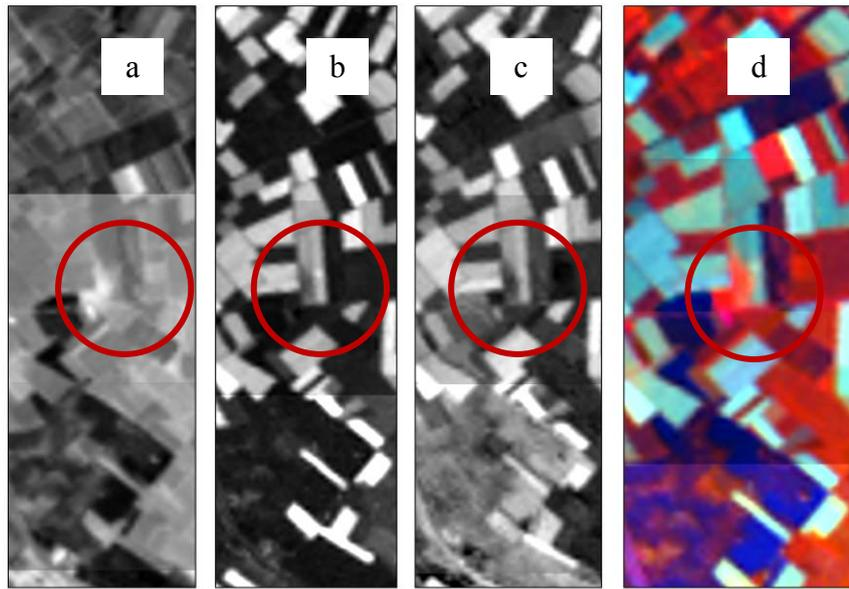
Figure 18: Tasseled Cap results for Nikaia 16 site (in red circle), (a) Brightness, (b) greenness, (c) wetness and (d) RGB of the first three components of the T-K algorithm.
