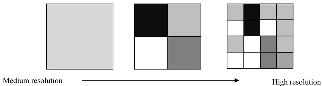
Figure 1: Example of a mixed pixel in different resolutions.
