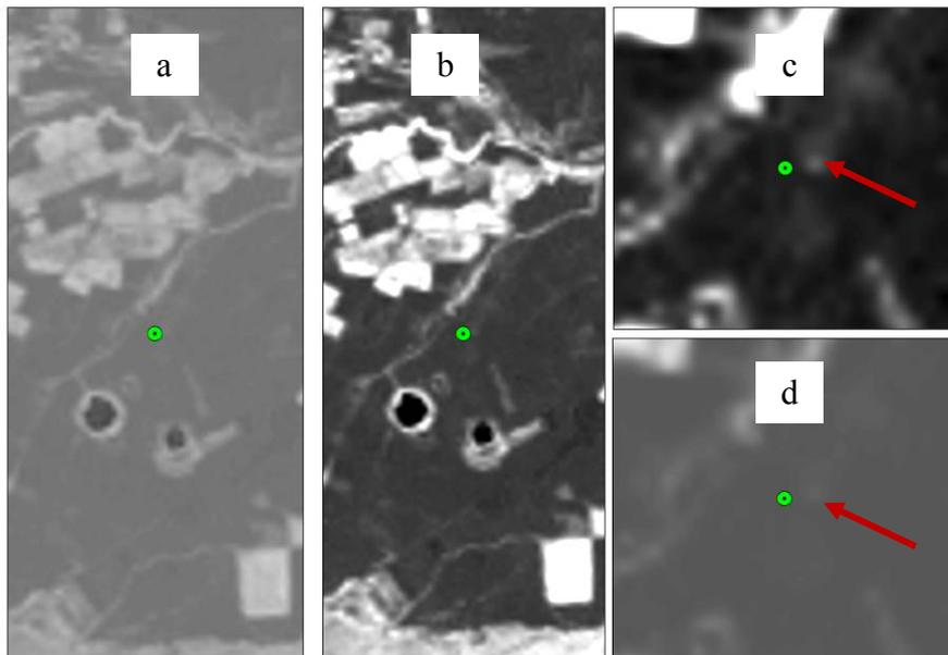
Figure 17: NDVI results for Zerelia site (in green circle). (a) raw satellite image without any radiometric enhancements, (b) satellite image with a linear max-min enhancement applied to all image, (c) max-min enhancement applied to the area around Zerelia and (d) modified max-min enhancement applied to the area around Zerelia. The magoula is indicated with the red arrow.
