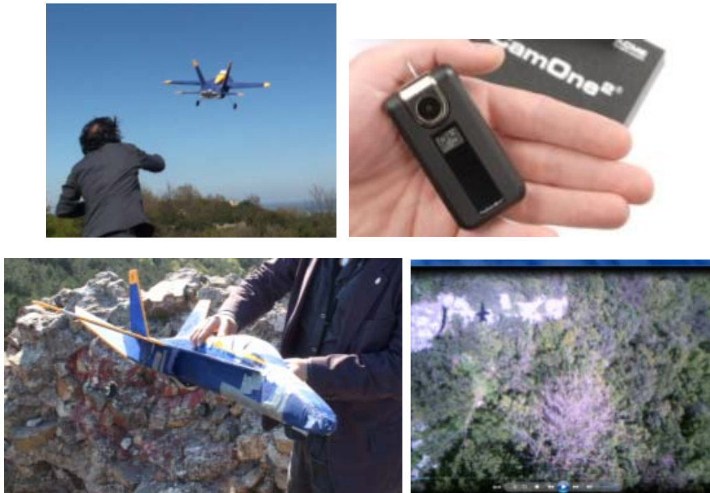
Figure 2: Flycam One 2 digital video camera attached to the model plane, and images obtained.
