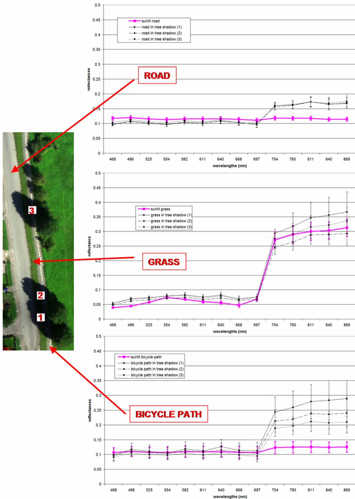
Figure 4: Selection of ROIs in three tree shadows over three ground materials for subset 2 (left side) and overlapping graphs of mean reflectance retrieval in the sun and shade for ICARE with standard deviation bar (right side).
