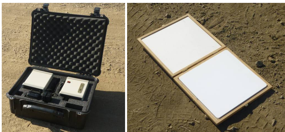
Figure 1: The GER 1500 spectroradiometer used in this study (left) and the calibrated spectralon panel (right).
