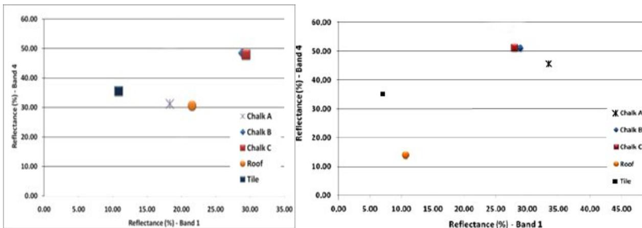
Figure 3: Scatter-plots of the different targets examined in this study for Band 1 – Band 4(humidity 0%) (left) and Band 1 - Band 4 of Landsat (humidity > 50%) (right).
