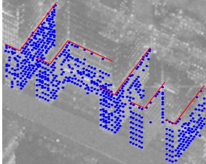
Figure 6: Selected base primitives (blue) and used building outlines (red) overlaid to the mean amplitude image of the data stack. The range direction of the sensor is bottom to top.
