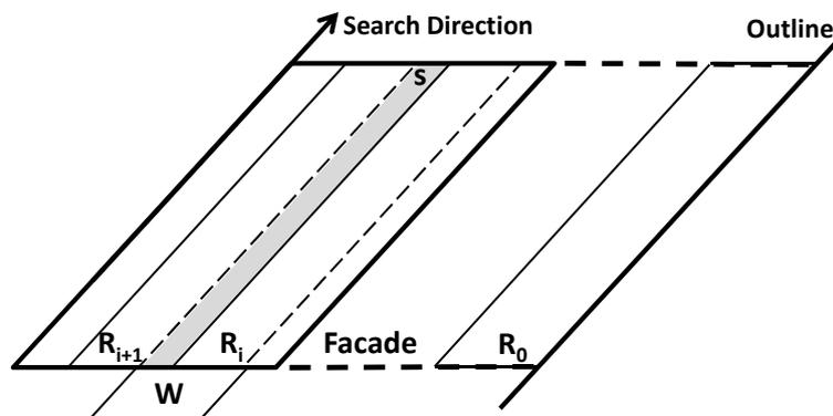
Figure 4: Preliminary search for rows along the façade. The first region  $R_0$  is defined at the outline of the façade. The other rows are constructed by consecutively shifting  $R_0$  in negative range direction. To ensure not to miss groups at the margins, the regions overlap.
