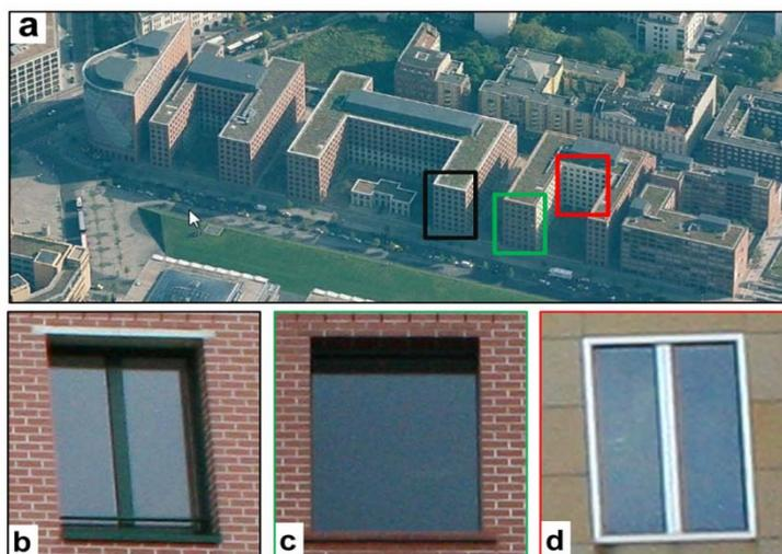
Figure 1: a) Oblique view aerial image of the building under investigation (© Microsoft® Bing™). The boxes mark areas, where the windows types shown in the close-up images b), c), and d) appear; b): Window type divided by a vertical and a horizontal structure. c): Plain window leading to the most point like amplitude patterns. d): Windows without a sill almost coplanar to façade. At those windows no PS could be detected.
