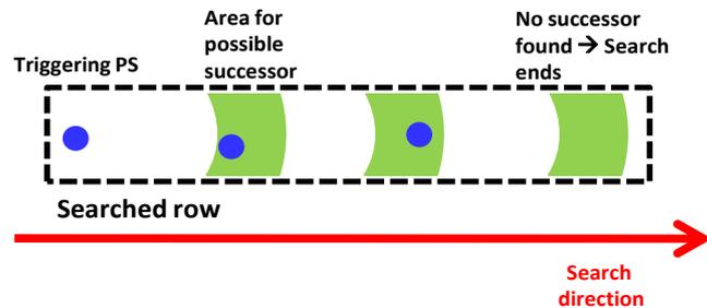
Figure 5: Illustration of the search process. Starting with a PS (triggering PS) a search area is defined. If a PS is found therein, it is added to the group and a new search area is defined. The process terminates if no successor is found.
