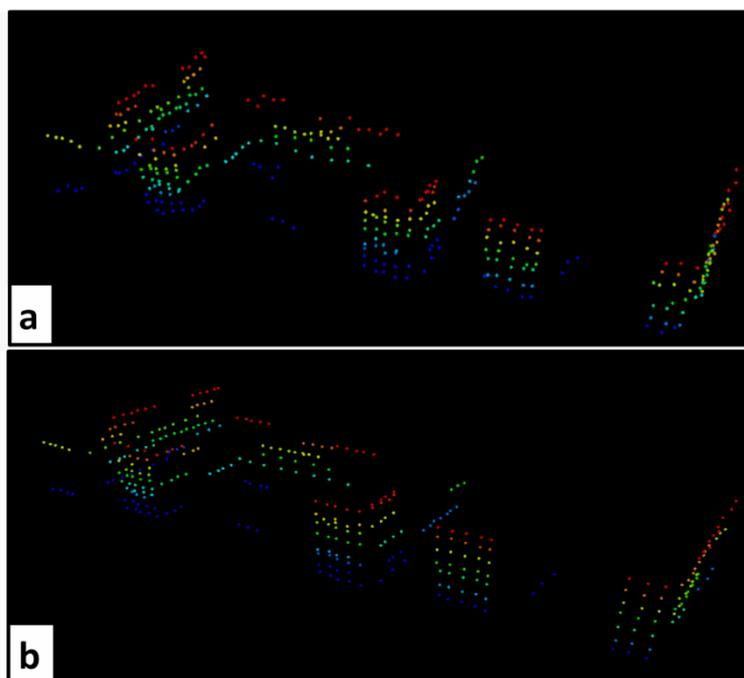
Figure 8: Geocoded PS using the originally estimated PS height (a) and the group mean (b) respectively. Since a height value is needed to determine the planimetric position of a PS, the grouping also improves the accuracy of the estimated PS position.
