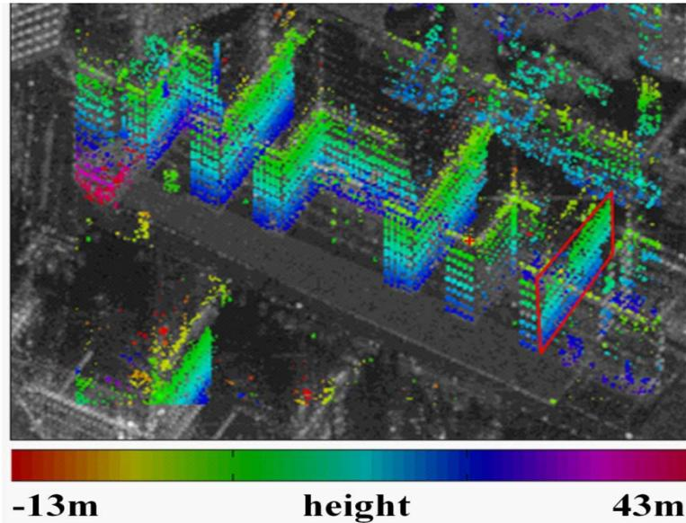
Figure 2: Result of a PS analysis for the considered test area. The color indicates the estimated PS height with respect to a reference point indicated by the red cross. The background image is the mean amplitude image of the used data stack. Points were selected if their temporal coherence is above 0.7.
