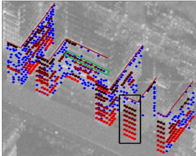
Figure 7: Result of the grouping algorithm. The selected PS are marked by dots, while the groups are indicated by lines connecting the dots. PS not been included in any group are shown in blue. Colors from black to light red indicate the mean height of the PS.
