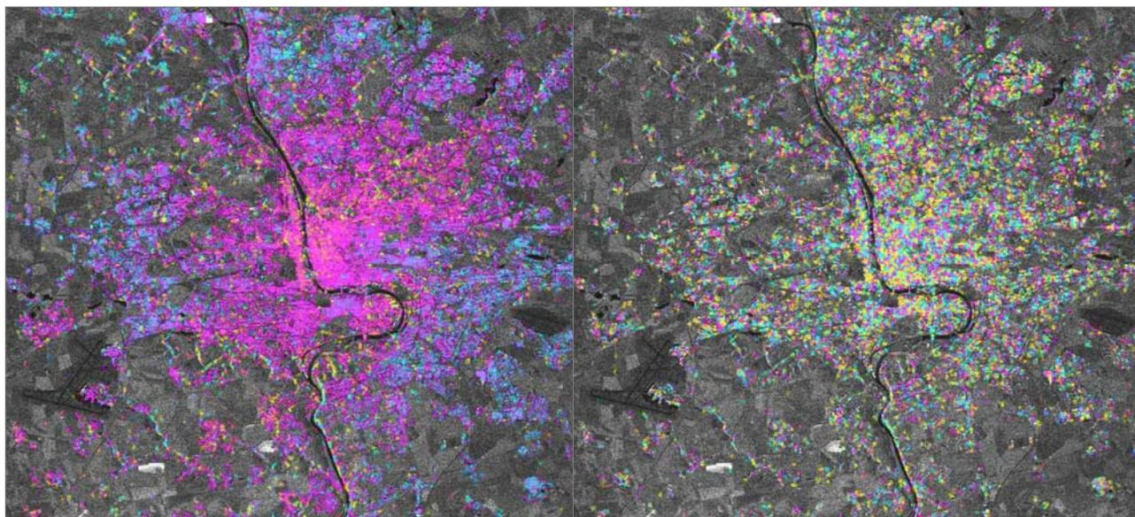
Figure 2: Differential interferogram obtained in an initial processing run for an interferometric pair with short perpendicular baseline (12 m, left). On the right the differential interferogram from last iteration for an interferometric pair with long baseline (803 m) is shown. One colour cycle corresponds to a  $2\pi$  phase cycle. It is clearly seen that the differential interferogram with the short baseline is smooth while the other is decorrelated.
