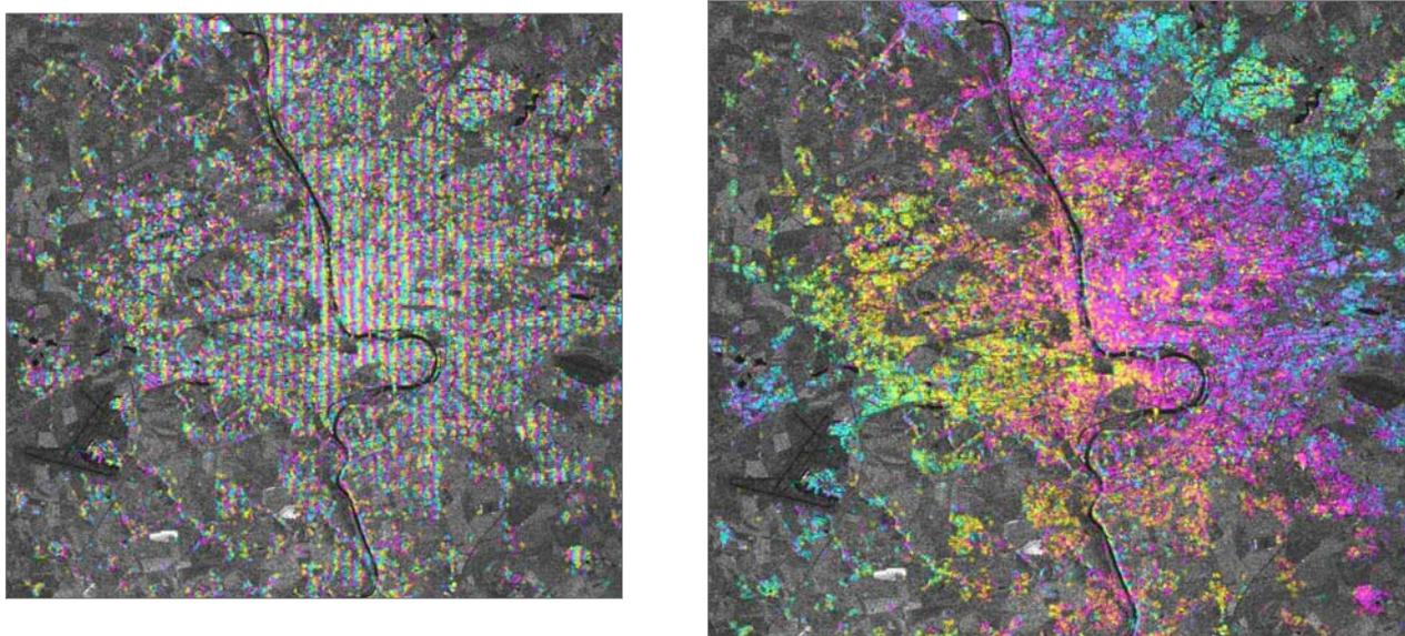
Figure 6: Example of the suspicious interferograms which will be further analysed. On the left there is an interferogram with erroneous flat-Earth phase subtraction. The precision orbits will be re-estimated for this pair and evaluated again. If the interferogram will not improve the scene will be excluded from the whole processing. On the right there is an interferogram in which the trend is clearly seen so it is candidate for the atmosphere influence removing.
