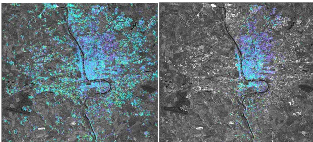
Figure 4: Relative linear deformation rate for the initial iteration cycle (maximum perpendicular baseline set to 350 m, left) and for the last iteration (all interferograms, right). One colour cycle corresponds to 0.05 m/year relative linear deformation rate. One can clearly see the decreasing amount of the processed points (relation to the baseline length) in the pictures.
