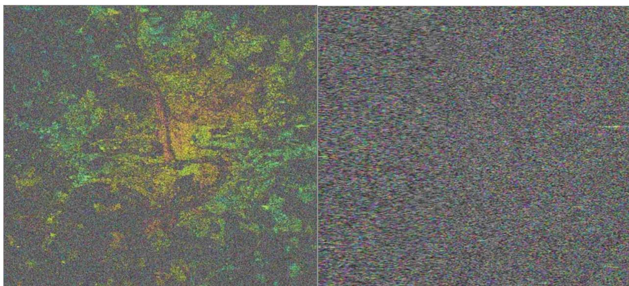
Figure 3: An example of the differential interferogram for the interferometric pair with short baseline (12 m, left) and for long baseline (802 m, right) from the conventional interferometry processing. The interferogram with long baseline is totally decorrelated and cannot be further processed.
