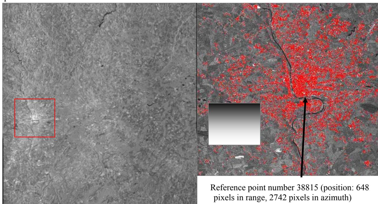
Figure 1: The whole scene (left) and the used cut (the red rectangle on the left of the scene covering Prague city area with candidate points (red dots, right). The images were displayed in multilook (1 in range and 5 in azimuth) for easier interpretation.
