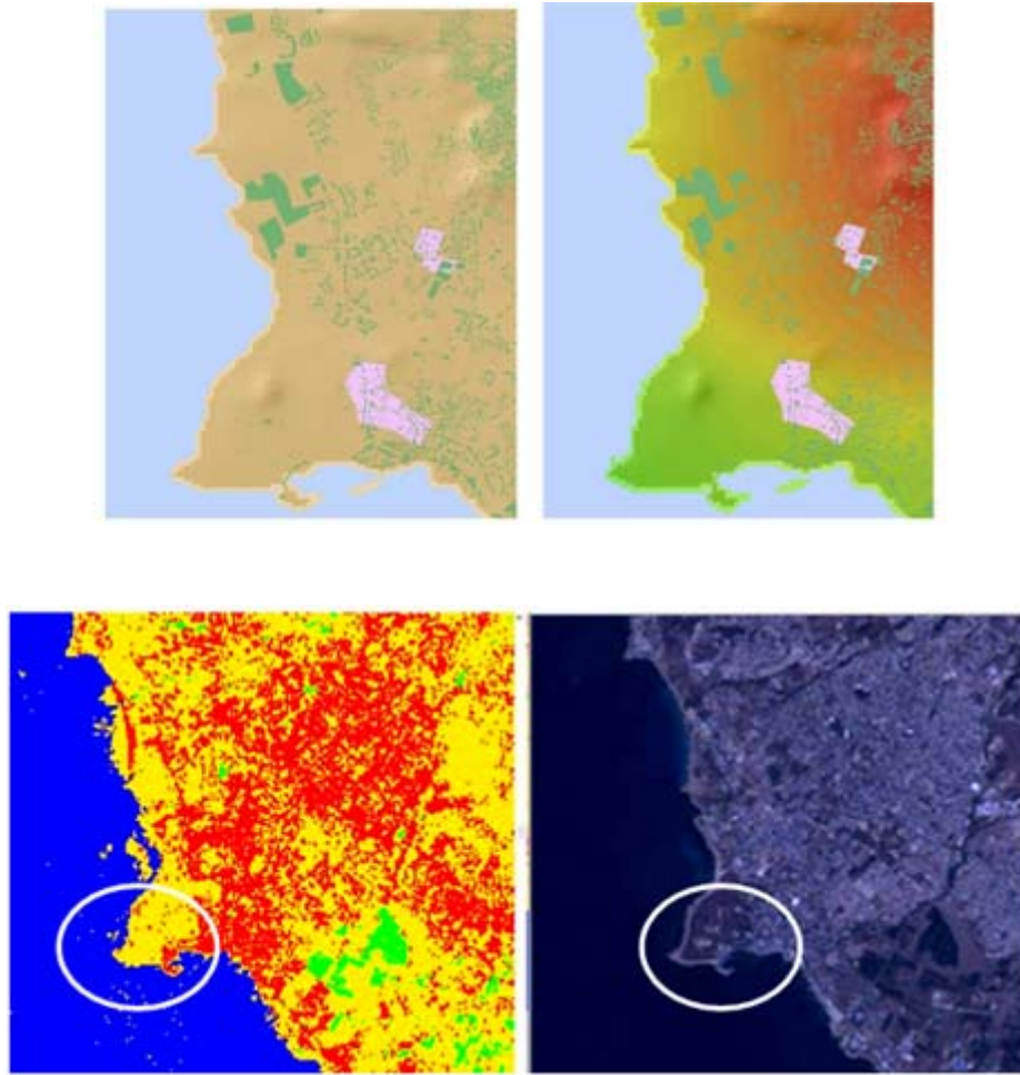
Figure 4: a) Overlay of the two different layers in GIS environment (green = 2008, purple = 1963). b) Density maps of urbanization for 2008 overlay with buildings of 2008 (green polygons) and buildings of 1963 (purple). c) Supervised Classification results at the “Nea Paphos” site using Landsat ETM+ image taken in 2009. With red colors the urban areas are indicated ; yellow=land; blue = water; green=irrigated/vegetated areas. d) Landsat ETM+ image taken in 2009.
