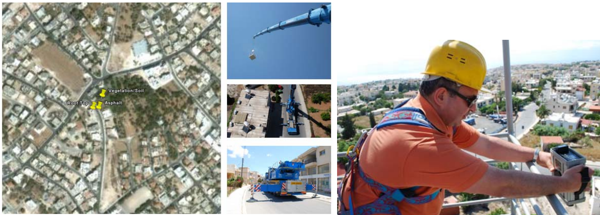
Figure 5: a) Study area and mobile crane b) Spectroradiometric measurements from the height of 40 m above the ground.
