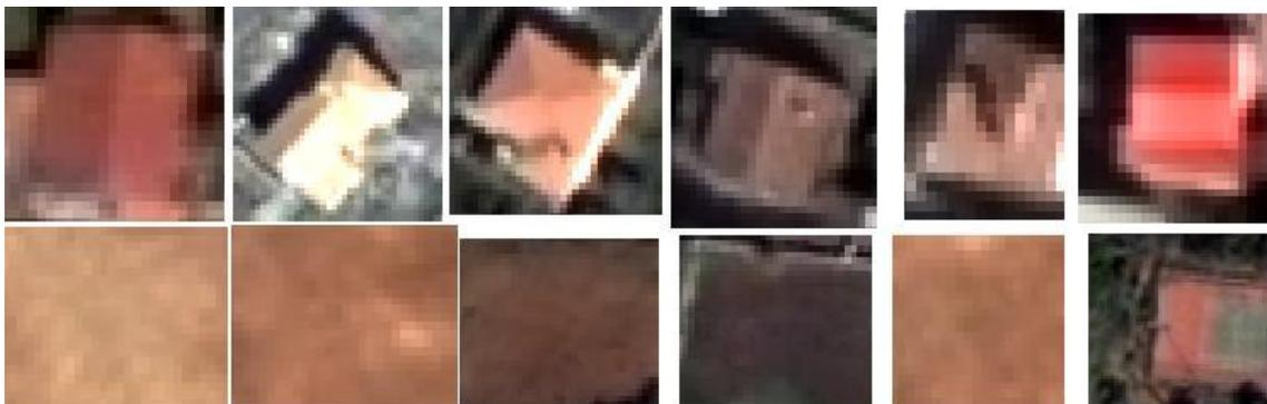
Figure 2: Spectral variety of tile roofs (top row) and background areas with very similar spectral characteristics (bottom row) of the study area.
