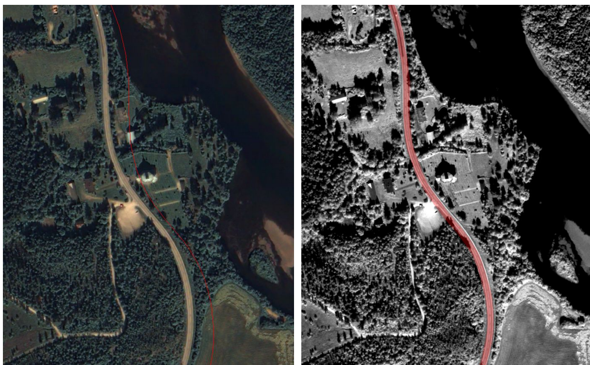
Figure 1: Left: road vector (red contour) directly overlaid on the (here: pansharpened) image. Right: resulting road mask (red layer) overlaid on panchromatic image.
