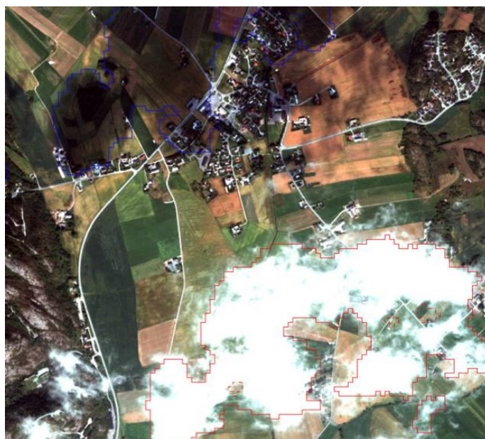
Figure 2: Result of cloud and cloud shadow classification. Clouds and cloud shadows are outlined in red and blue, respectively.
