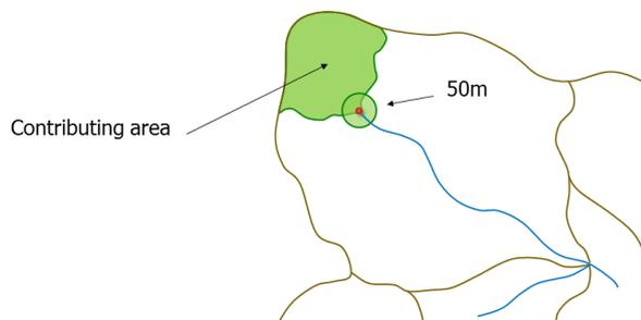
**Figure 4.** A 50m-buffer around a spring overlaid on its drainage area compose the area to be protected.
