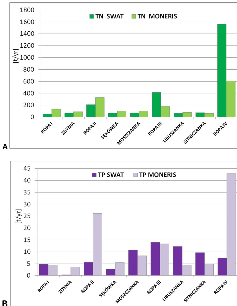
**Figure 7.** Diagrams illustrating loads of nitrogen (A) and phosphorus (B) derived from SWAT and MONERIS models
