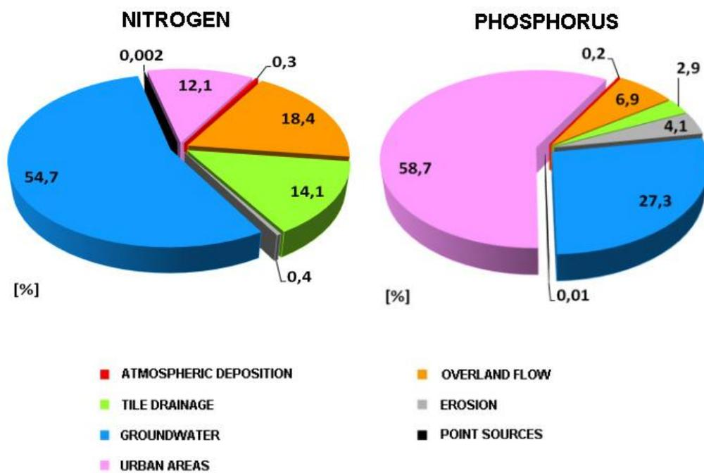
**Figure 6.** Sources of nitrogen and phosphorus emission in Ropa catchment
