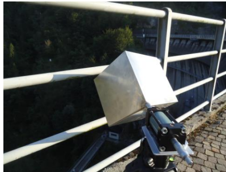
Figure 1. Corner reflector used to assess the precision and accuracy of GBSAR displacement measurements.
