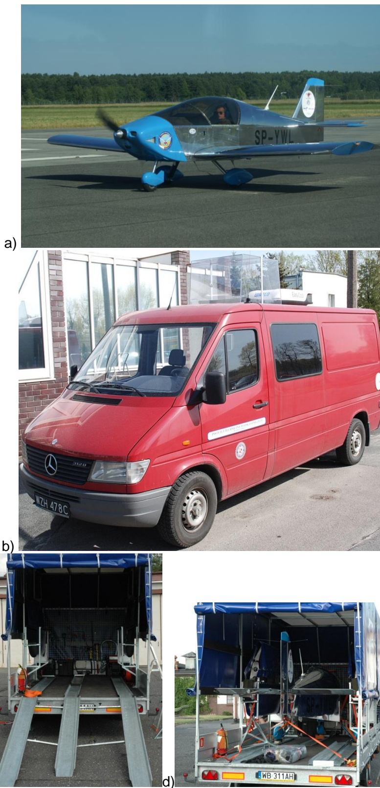
Figure 1. Elements of the Flying Laboratory a) Sonex airplane b) mobile ground platform, c) and d) special trailer for carrying Sonex airplane – c) empty, d) with loaded airplane.
