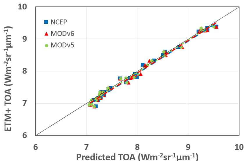
Figure 2: Plot of ETM+ b6 radiance versus the VC-based radiance (predicted). Results are provided for three atmospheric profiles: MOD07 product (version 5 and 6) and the NCEP reanalysis profiles.
