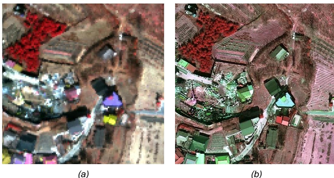
Figure 2: Input data for this study (a) CASI displayed in 801.1 nm, 643.3 nm, and 557.2 nm and (b) DMC images displayed in NIR, red, and green spectral range as RGB channel
