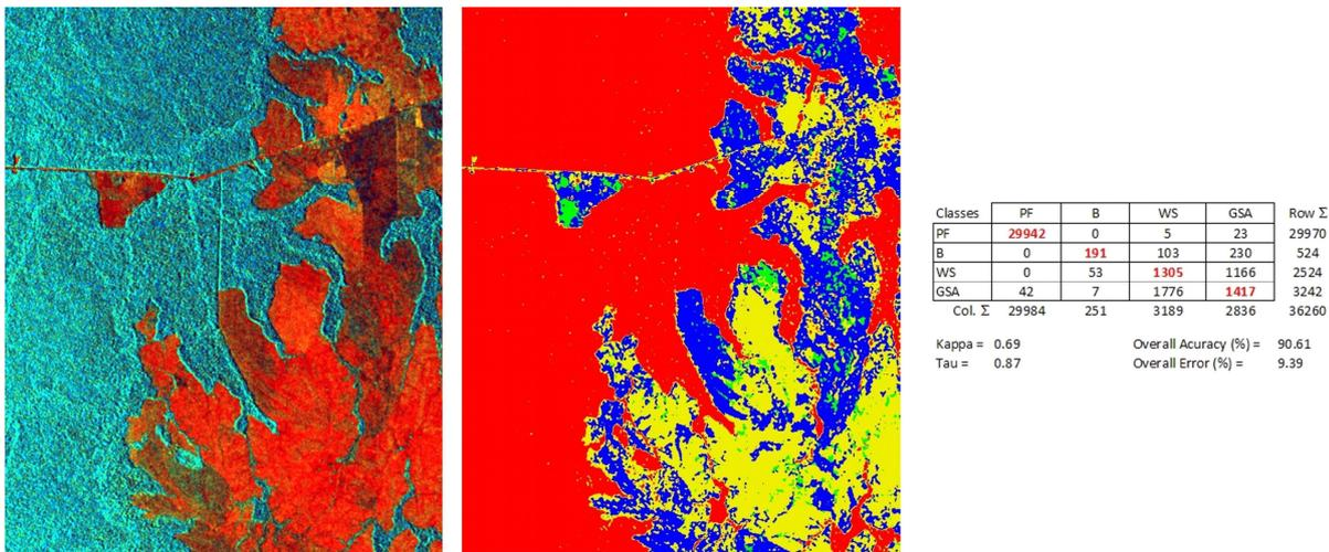
Figure 1. (a) Color composite image combining the InSAR coherence (red) + backscatter (green) + ratio of coherence/backscatter (blue) derived from Cosmo-SkyMed (Stripmap mode); (b) ICM land cover classification with Primary Forest (PF) in red, Burned area (B) in green, Wooded Savanna (WS) in blue; Grass/shrub Savanna Area (GSA) in yellow; (c) the classification performance matrix.
