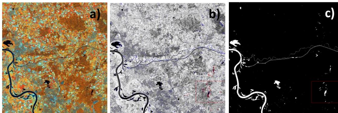
Figure 2. a) RapidEye infrared combination, b) low albedo and c) water mask, according to estimated threshold. Ruhr area (Germany), 26.07.2012.
