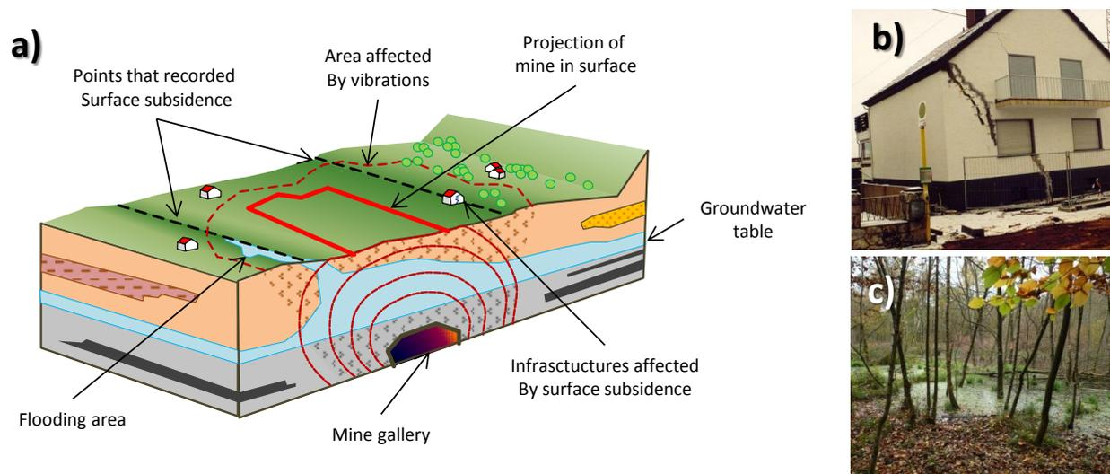
Figure 1. a) 3D scheme of changes in substrate and groundwater dynamics around a gallery mine. B) Damages caused in infrastructures and c) the environment (flooding) due to ground movements.
