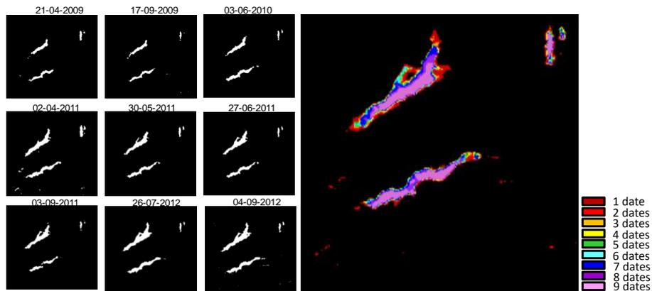
Figure 3. Left: water masks for a known flooded area in Kirchheller Heide for the period 2009-2012. Right: results of the change detection using those nine RapidEye water masks.
