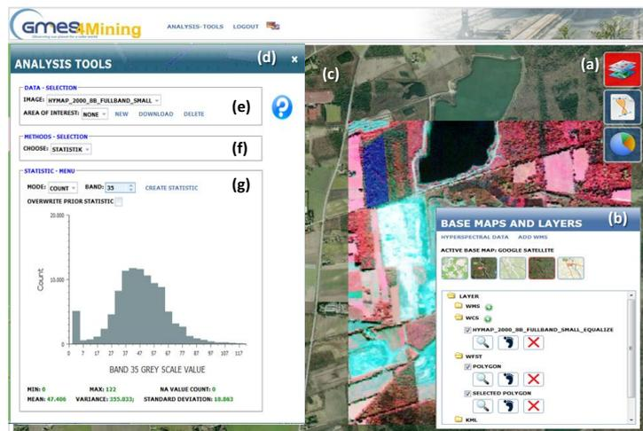
Figure 4. Elements of the geoportal: (a) key access to different layer managers and functions, (b) layer manager window, (c) displayed raster data, (d) Dialog window for methods and analysis, (e) data selection pull-down list, (f) method selection pull-down list, and (g) Results/Statistics window.
