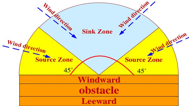
Figure 3: Schematically effect of wind direction and determination Sink Zone and Source Zone near obstacle
