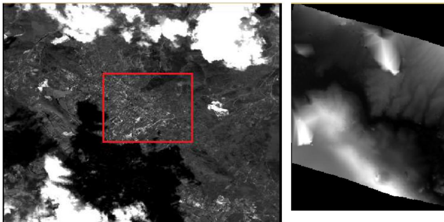
Figure 8. The selected area for DSM Extraction and the result obtained from real stereopair (Paganica)
