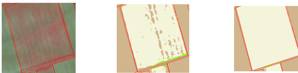
Figure 1. Example of crop classification homogenisation using the 2012 crop parcels (RPG): Crop-parcels overlain on the 01/04/2012 Pléiades image (left), the initial crop classification (centre) and majority crop allocation to parcels
