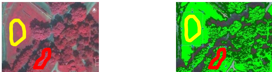
Figure 1. Difficulty in discriminating between low-lying (yellow) and high (red) vegetation signatures. A spectral overlap is seen between low-lying (bright green) and high vegetation (dark green) areas.
