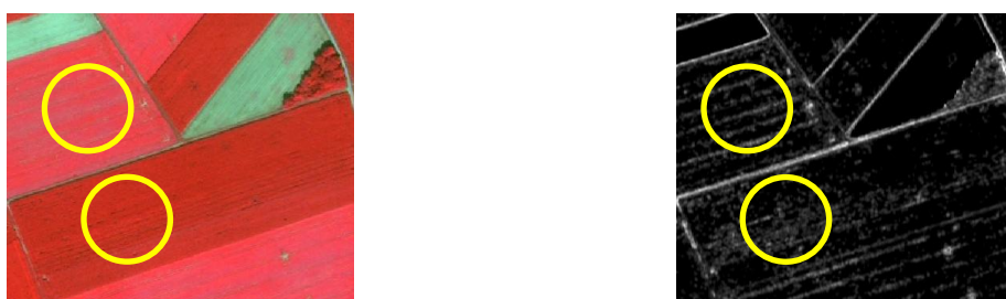
Figure 3. Texture index highlighting a copse, agricultural paths and tractor paths in fields (yellow circles) – standard Pléiades NIR colour composite on left, texture index on right.
